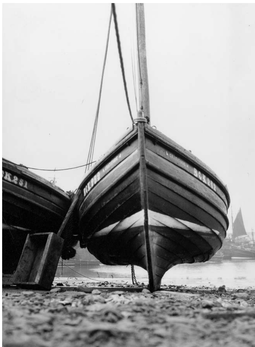
This photograph shows so clearly the hollow floors and the sharp turn to the bilges of the now well-known scaffie yawl Gratitude BCK252. She is photographed at Portnockie on the Moray coast c1936. (NMM, Oliver Hill Collection, neg no P75448)
